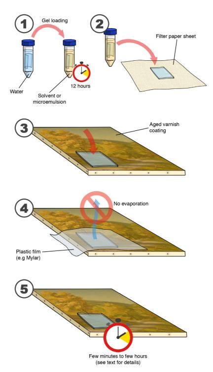
**Figure 2a.** Application of Nanorestore Gel® Dry (loaded with solvents or Nanorestore Cleaning® formulations) for the removal of polymeric coatings or varnishes.
