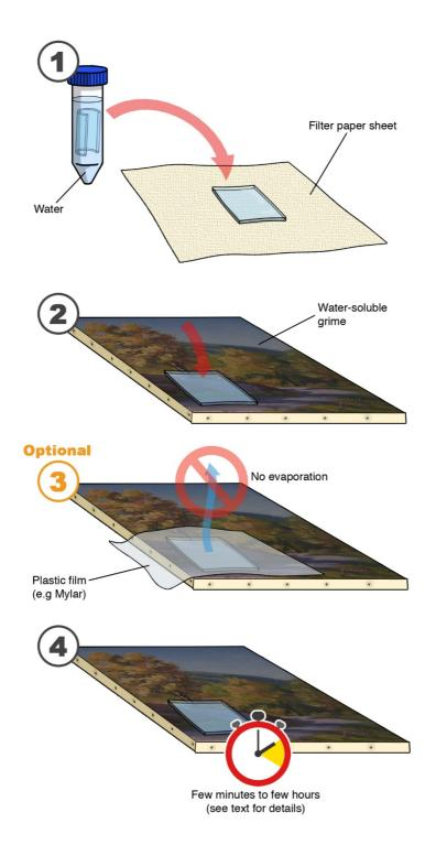
Figure 1a. Application of Nanorestore Gel® Dry for the removal of hydrosoluble dirt.
