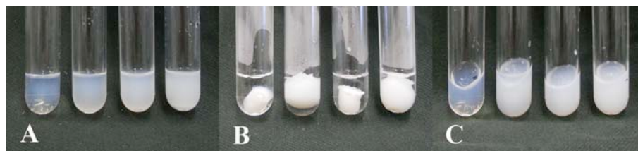
Figure 2: PNIPAM hydrogels with increasing HAP content going left to right at A) 20 °C, B) after heating at 50 °C and C) cooled from 50 °C to 20 °C.
